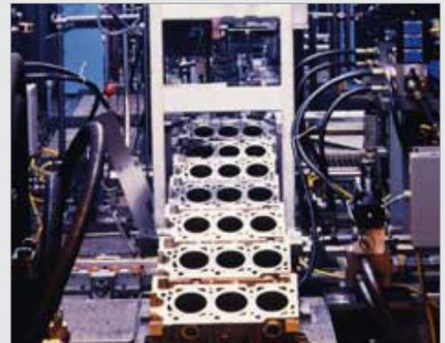
In the crankshaft bore operation, all stock is removed in a single pass process simultaneously. Much like the cylinder bore ream process, the tool passes through the journals at an appropriate rate that provides excellent gore geometry and final surface finish.
